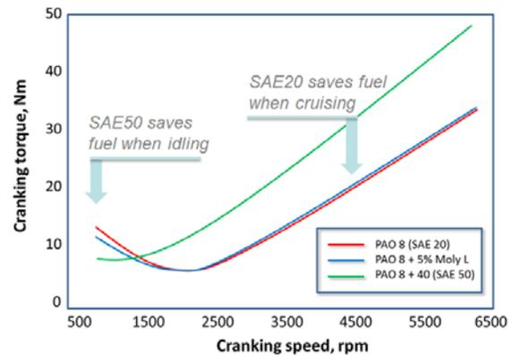
**Figure 3** / Friction torque measurements carried out for a common i4 production engine using model lubricants to mimic 0W-20 and 5W-50 motor oils.
