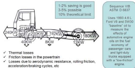
**Figure 2** / Energy losses in cars and typical fuel economy figures achievable in Sequence VIB due to oil upgrade.
