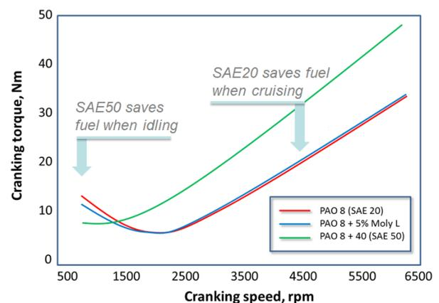
**Figure 2** / Friction torque measurements carried out for a common i4 production engine using model lubricants to mimic 0W-20 and 5W-50 motor oils.
