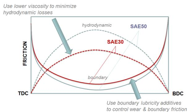
**Figure 1** / Standard practice: Reducing engine friction by using a lower viscosity oil in combination with boundary lubricity additives.
